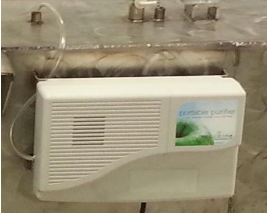
An ozone generator is included and mounted to the front of the recycler. A ¼" feed line and air stone is installed in the the second chamber and should be positioned so the air stone is sitting 2/3 of the way down in the tank. Ozone kills bacteria, molds, mildew and other odors. The generator should be run at all times. This generator is compressor driven and operates on 120 volt .15 amps.
